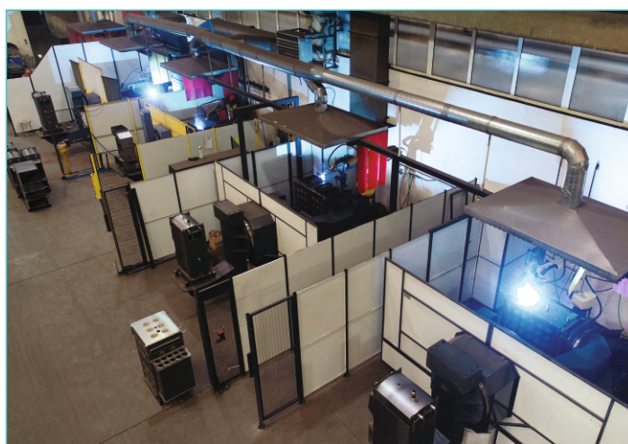
Robotic welding of the boilers
