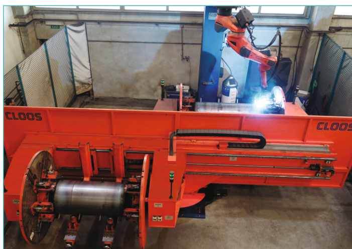
Robotic welding of stainless steel water heaters
